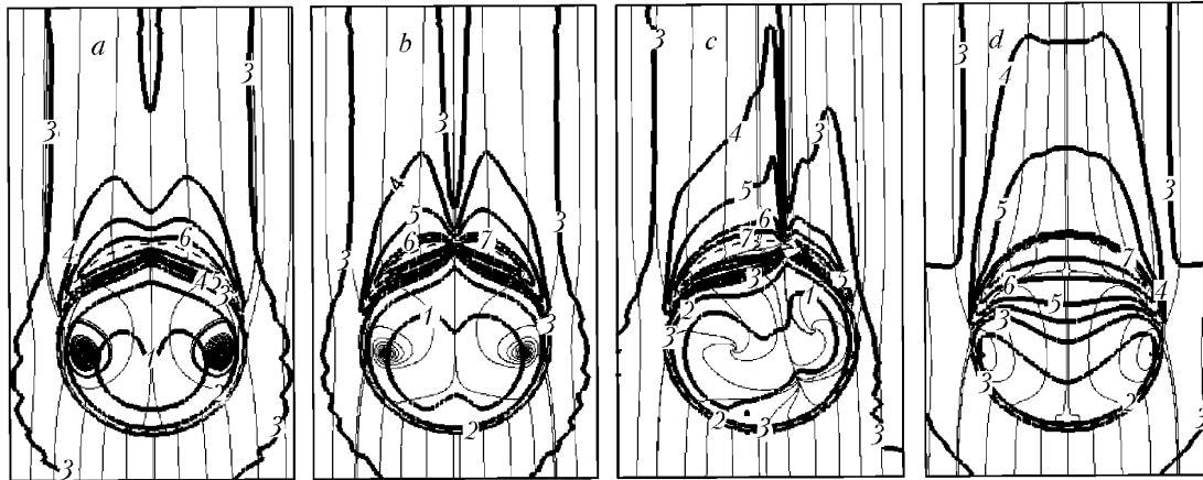
Fig. 5. Influence of Re on the patterns of relative-heat-transfer isolines including fluid-spreading lines: Re = 3 \cdot 10^3 (a), 5 \cdot 10^3 (b), 9 \cdot 10^3 (c), and 2 \cdot 10^4 (d). The lines to which numerical values are assigned correspond to Nu/Nu_{pl} = 0.2 (1), 0.6 (2), 1 (3), 1.2 (4), 1.4 (5), 1.8 (6), and 2.2 (7).
